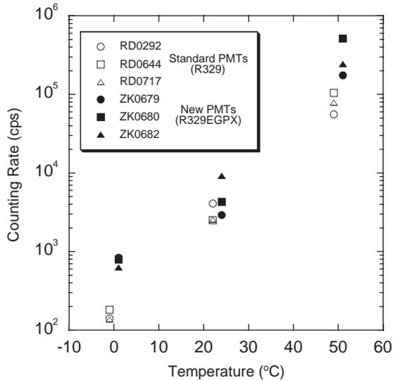
Fig. 12. Background noise counting rates as a function of the temperature in the darkcurrent measurement. The threshold voltage value corresponding to 0.5 p.e.. The open symbols denote the results for the original PMTs, and the closed symbols are for the new ones.
