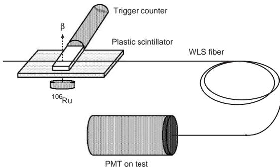
Fig. 3. Experimental setup for measuring the number of photoelectrons.
