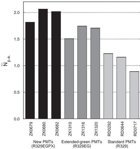
Fig. 5. Averaged numbers of photoelectrons obtained with the new PMTs (ZK0679, ZK0680, ZK0682), the extended-green ones (ZK1310, ZK1316, ZK1320) and the standard ones (RD0292, RD0644, RD0717).
