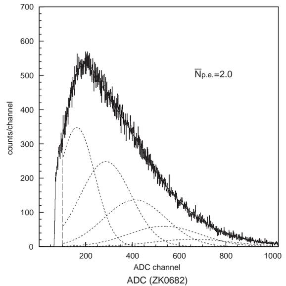
Fig. 4. Typical ADC spectrum obtained with the new PMT. The solid curve is the result of the fit described in the text. The dotted curves are decomposed Gaussians for  $N = 1, 2, 3, 4, 5$ .
