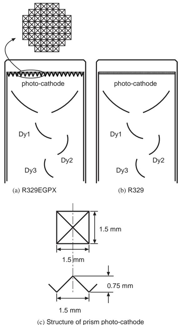
Fig. 1. Schematic structure of (a) the new PMT (R329EGPX); (b) the standard PMT (R329). The photocathode of the new PMT has 827 prisms on its surface. The thickness of photocathode material is the same for both PMTs; (c) structure of each prism.
