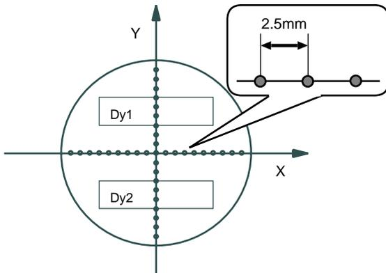
Fig. 7. Fiber positions of photon incidence in the measurement of TTD and uniformity.
