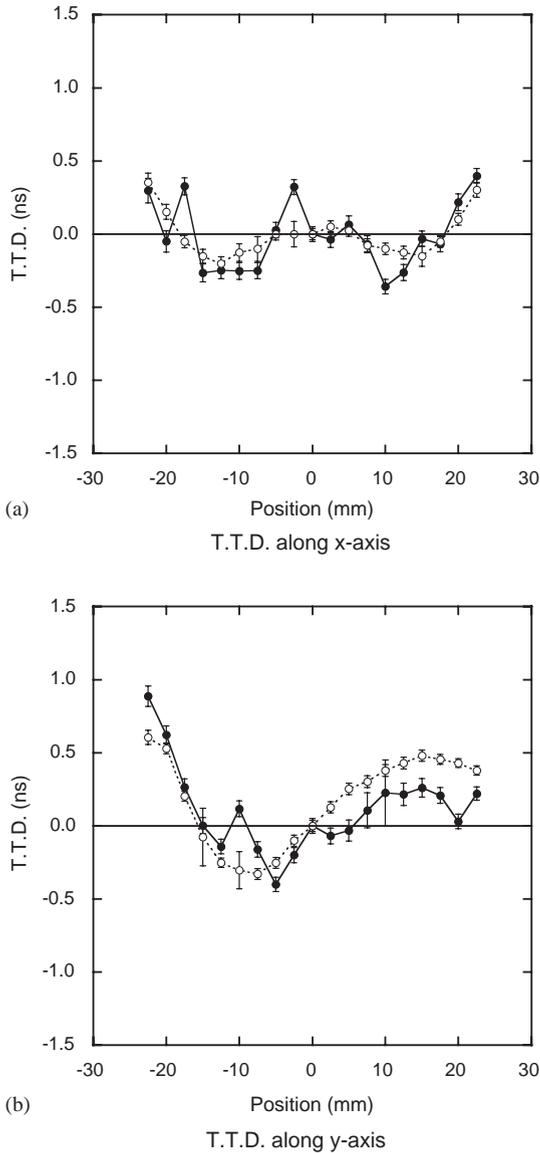
Fig. 9. TTD along (a) x-axis and (b) y-axis for the standard PMT (open circles) and the new PMT (closed circles). The PMTs are operated at 2.5 kV. The error bars are the root-mean-squares of the TDC distributions.
