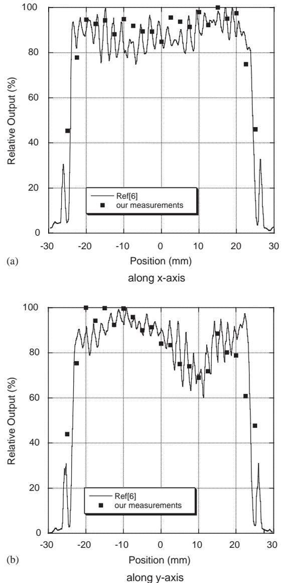
Fig. 6. Position dependence of the sensitivity for the new PMT (R329EGPX). The definition of the axes is the same as described in Fig. 7. The solid lines represent the data taken by Hamamatsu Photonics K.K. at 420 nm. The closed squares represent our data for the fiber readout with the WLS fiber of 1 mm in diameter.
