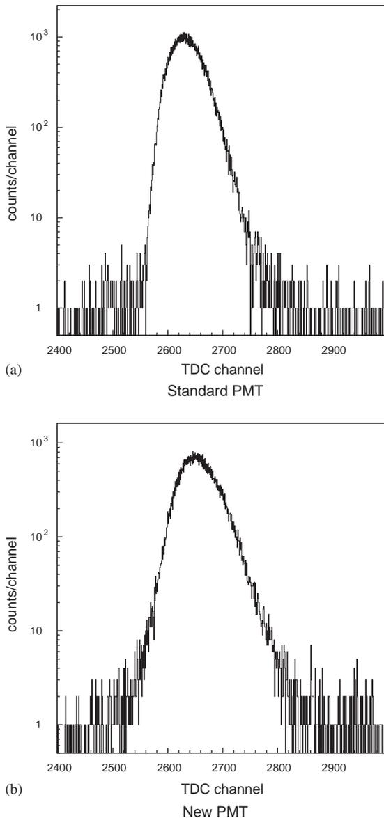
Fig. 11. TDC distributions obtained with (a) the standard PMT and (b) the new PMT. The scale of the horizontal axis is 25 ps/channel.
