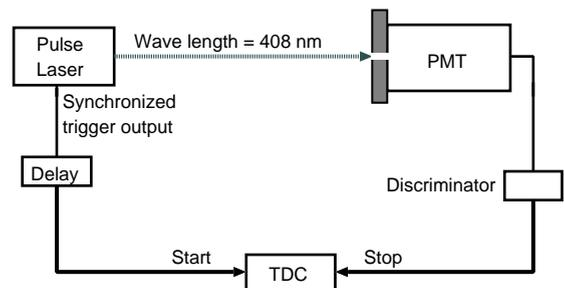
Fig. 8. Setup for the TTD measurement.
