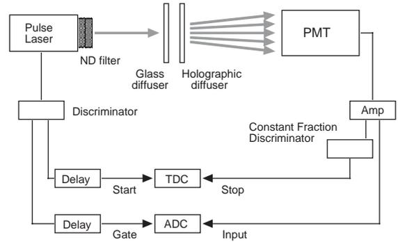
Fig. 10. Setup for the TTS measurement.
